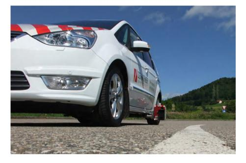
ZDR 6020 Dynamic retroreflectometer  $R_L$  for all types of road markings at normal traffic speed without obstructing the traffic.
