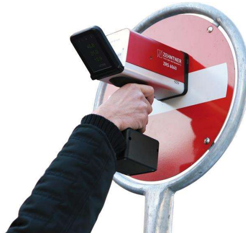
Figure 3. Zehntner's ZRS 6060 Retroreflectometer for traffic sign retroreflection measurements
