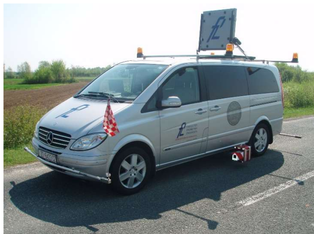
Figure 1. Department's measuring vehicle with Zehntner ZDR 6020 Retroreflectometer
