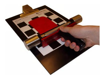
dismantle the apparatus after every print proof and clean it carefully with a suitable solvent
