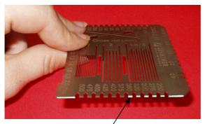
The picture shows that the tooth 350  $\mu$ m is the last tooth which has been wetted by the coating and the tooth 375  $\mu$ m is not wetted. The wet film thickness is between 350  $\mu$ m and 375  $\mu$ m.
