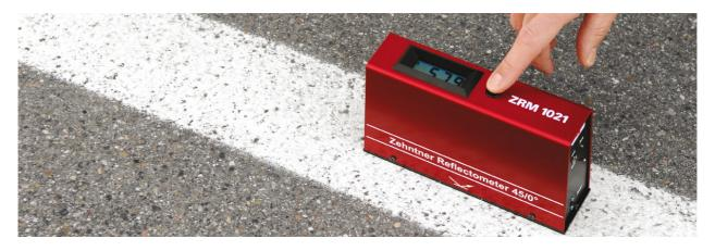
The  $\beta$  value is calculated by dividing the value of the instrument by 100: If you receive with our instrument for example the value 78.0, the  $\beta$  value is 0.78. So when the instrument measures 57.9 the  $\beta$  value is 0.579, when it measures 60.0 the  $\beta$  value is 0.6.
