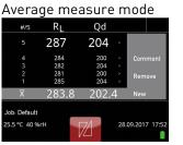
In average measure mode you can delete a single value (e.g. an outlier) by tapping on this value. To comment on a series of measurements tap on the average value at the bottom. An editing menu will open next to the list. Tapping on "Remove" will delete the whole series of measurements. To start a new series of measurements tap on "New".
