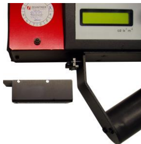
Fig 5: Barcode reader dismantled
