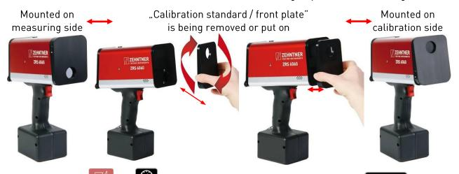
Press the symbol and calibrate to open the calibration function. By pressing trigger the calibration. After the calibration you get a message that the calibration was
