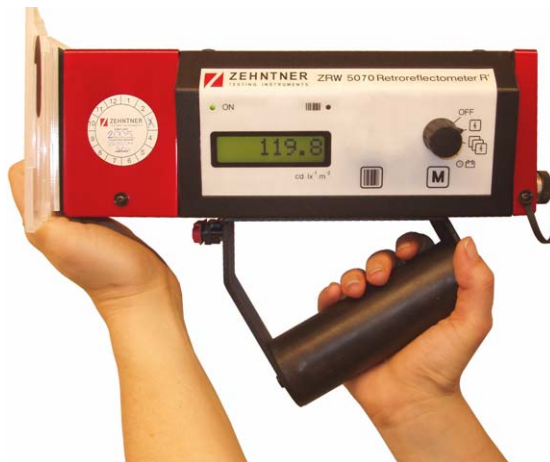
Correct Measurement alignment
