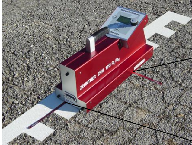
Figure 20 Position of the measuring instrument and the scales of the rulers after the fourth and last measurement
