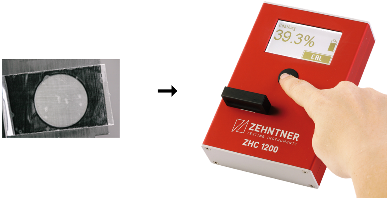
Determination of chalking with chalking tester (Zehntner ZHC 1200)
