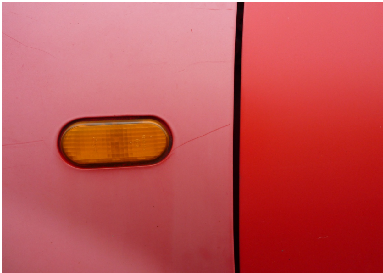
An example for chalking on a car: car wing (left) affected by chalking compared with a new door (right) (Wikipedia)
