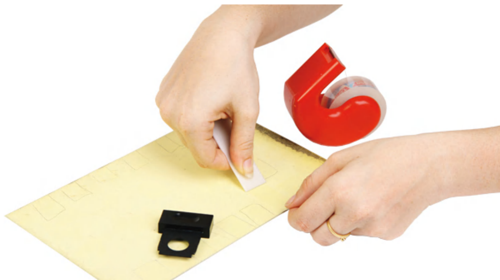
Transferring chalking particles to adhesive tape
