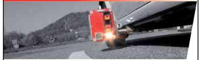
ZDR 6020 Dynamic Retroreflectometer R L measures the night visibility of road markings handheld precision at traffic speed up to 150 km/h (93 mph)
