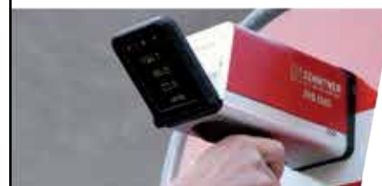
ZRS 6060 Retroreflectometer R A measures the night visibility of road signs and warning clothes triple angle measurements with colour touchscreen
