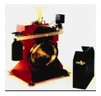
The machine consists of a road wheel, rotating at 320 rpm, to the periphery of which are clamped 14 specimen holders. A solid rubber tyred wheel is positioned vertically above the road wheel, and loaded to exert a force of 725 N.
