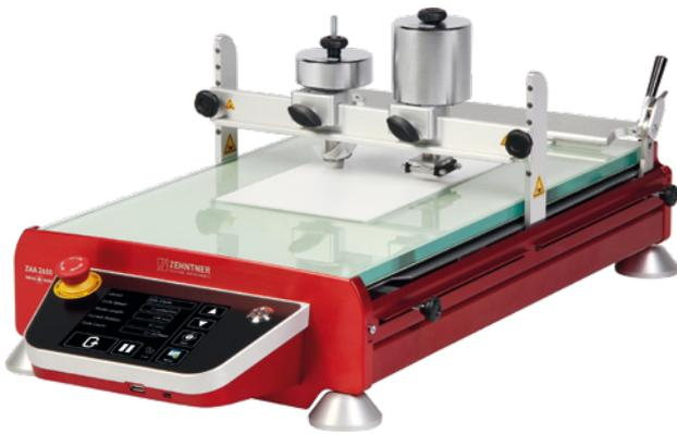
Up to 4 crockmeter tests can be carried out at the same time /
